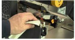
Printheads typically fail because of the fast heating and cooling process used as printing elements switch on and off when they pass over a paper or printing ribbon. Another major reason for breakdown is the pressure that is applied to fine tune print quality.
