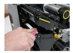
Before deciding to replace a printhead, make sure it has been properly cleaned. When you do clean your printhead, remember to also wipe your platen roller. A platen roller serves as a solid surface to which the label and ribbon are pressed and it pulls labels through the printer. As it wears, it becomes shiny and may cause labels to slip. By keeping it clean, you extend its life and help achieve good print quality.
