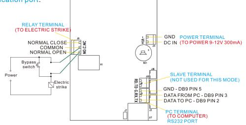
**DC IN TERMINAL** - Connect to the 12V DC power for the reader. **SLAVE TERMINAL** - Connect to a slave reader. **PC TERMINAL** - Connect to a PC for setup and database. **RELAY TERMINAL** - SPDT relay output for electric strike control.
