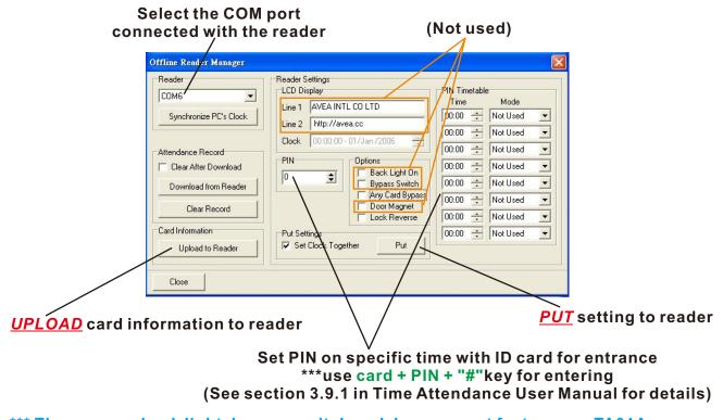
\*\*\* There are no back light, bypass switch and door magnet features on TA01A.
